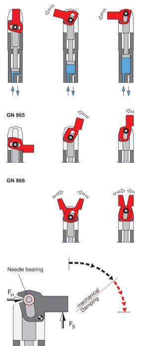
These pneumatic fastening clamps (Patent results) ) are used for clamping, holding, gripping and positioning of workpieces in jigs and handling systems.
