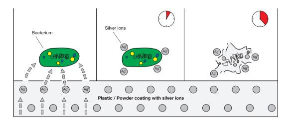
The antimicrobial effect of the additive is not reduced by repeated cleaning with soap or solvent. Even at sterilization temperatures the effect is not lost.
